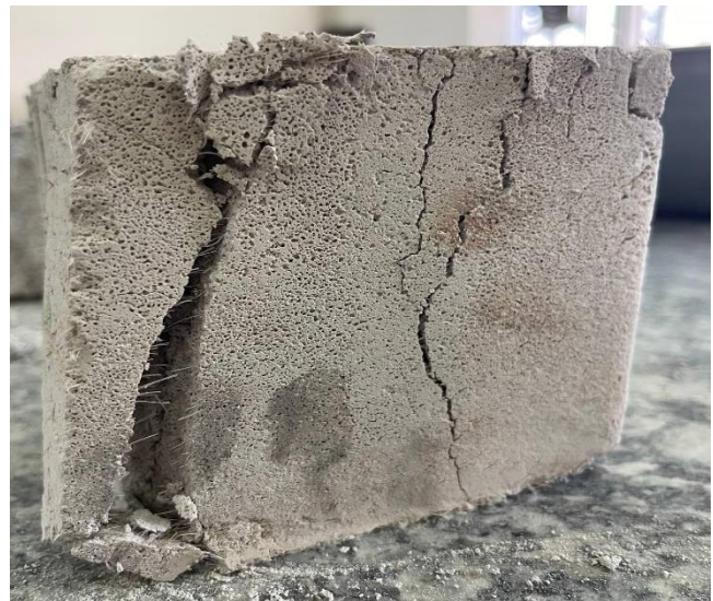
Figure (11): The sisal fibers act as bridges within AAC
