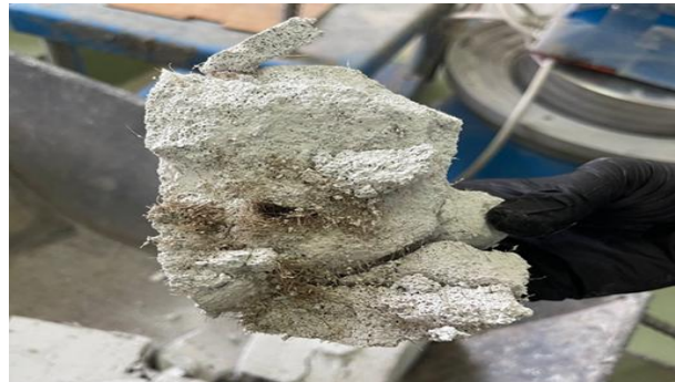
Figure (7): The fiber clumping within the AAC sample.
