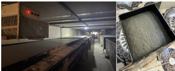
Figure (3): (a) the molds, (b) the drying room, and (c) the green cake of AAC
