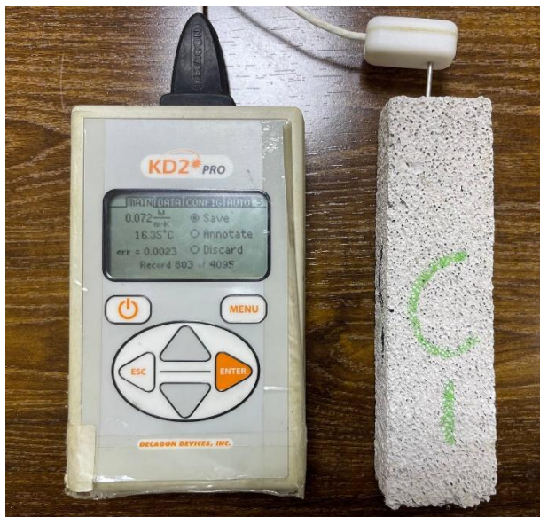
Figure (13): The sample of AAC under the thermal Conductivity test
