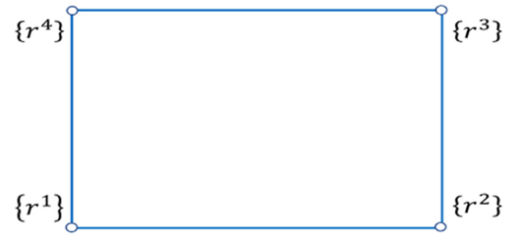
Figure 9. Quadrilateral element with four nodes and seven degrees of freedom per node [31].
