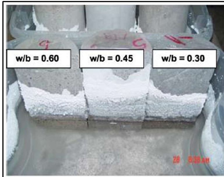
Figure 1: Salt efflorescence of concrete cylinders partially immersed in a sodium sulphate solution (Nehdi and Hayek, 2005).
